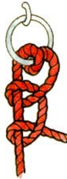
Round turn and two half hitches
